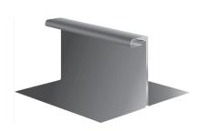
Handcrafted standing seam systems have a long tradition. Panels run vertically up the length of the roofs and are lock-seamed together by hand or simple machinery. The system is generally used for small to medium size roofs (up to 2.000 sqm). Larger surfaces are mostly equipped with the automated standing seam lock systems.
