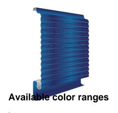
25/250 refers to the depth of the panel (25 mm) & the height (200 mm). Micro lining of the panel surface is done for aesthetic reason or to enhance the structural strength. Plank profiles are continuously manufactured and cut to length after the roll forming process. They come in many different shapes and sizes. For structural performance reasons application should not exceed 6.000 mm. Application can be done vertically and horizontally.
